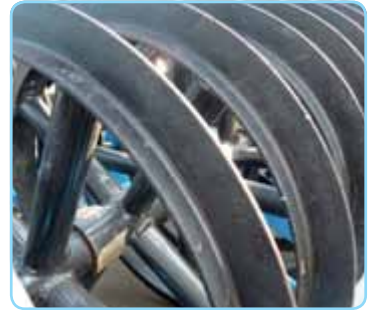
T-ring roller \phi 600 mm / T-Ring Walze \phi 600 mm / Rouleau T-RING \phi 600 mm
