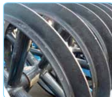
T-ring roller \phi 600 mm / T-Ring Walze \phi 600 mm / Rouleau T-RING \phi 600 mm
