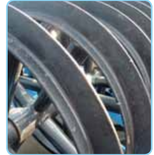
T-ring roller \phi 600 mm / T-Ring Walze \phi 600 mm / Rouleau T-RING \phi 600 mm
