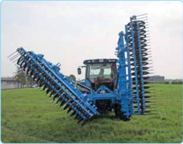
hydraulic folding to vertical position / Zusammenklappung System V / machine repliable en V
